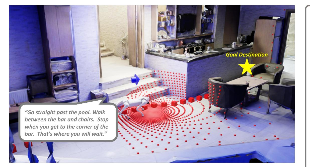
**Environment:** Nvidia Omniverse Isaac Sim Simulator **Agent**: Unitree Go2 Quadruped Robot **Perception**: RGB-D Camera Images
